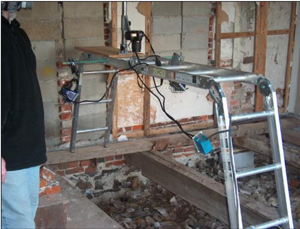
Figure 5: Scaffold with Lights and Camera Used for Photography.
